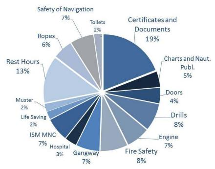
Most Frequent Detainable Deficiencies Detected During PSC Inspections in Romanian Ports
